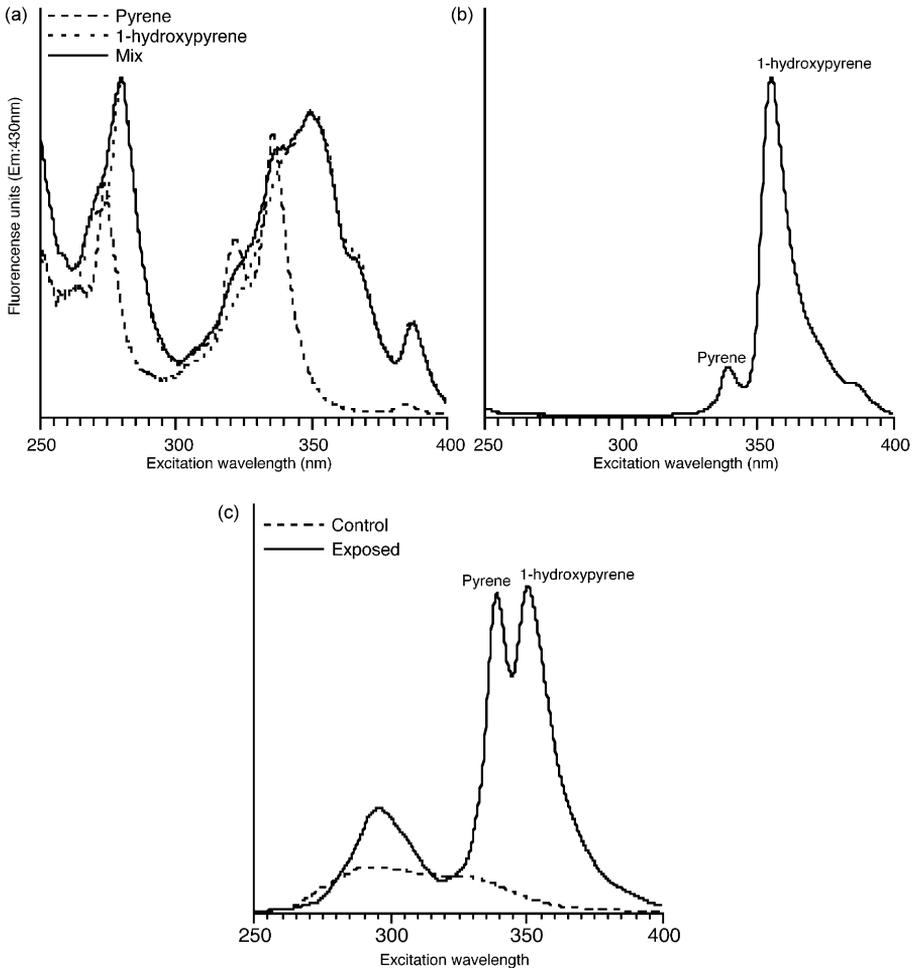
Fig. 1. Fluorescence spectra of pyrene and 1-hydroxypyrene. **a:** Traditional fluorescence spectrum of pyrene (30 ng/ml) and 1-hydroxypyrene (10 ng/ml) standards scanning the excitation channel while measuring emission at 430 nm. **b:** Synchronous fluorescence spectrum (SFS,  $\Delta\lambda = 34$  nm) of the same mixture of pyrene and 1-hydroxypyrene. **c:** SFS spectrum ( $\Delta\lambda = 34$  nm) of tissue extract from *Nereis diversicolor* exposed to pyrene contaminated sediment.
